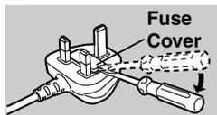
1) Remove the Fuse Cover with a screwdriver.
