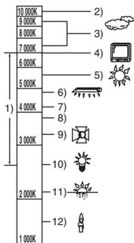
Outside of the effective range of Automatic White Balance Adjustment, the image will become reddish or bluish. Even within the effective range of Automatic White Balance Adjustment, the Automatic White Balance Adjustment may not function properly if there is more than one light source. In this case, adjust the White Balance.
